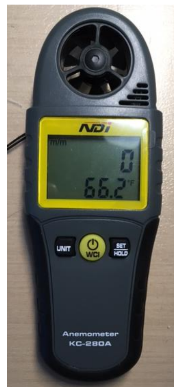
Anemometer- measures air velocity
